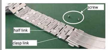
②Lift up the A link of the half link and clasp link to remove it.
