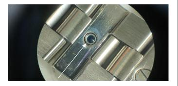
Apply it evenly inside the female thread. (In the photo A link was removed to make it easier to see)
