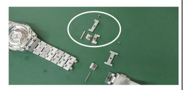
⑥Attach the Clasp link's C link with the B link on the bracelet side, and pass through the pin.
