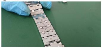
(13) Finally, put back the spring bar removed in (1) and complete.
