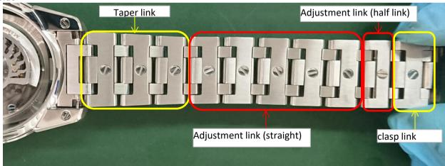
When adjusting the links, increase or decrease the links in the <u>red</u> frame area, and avoid removing the <u>yellow</u> frame area as much as possible. If you have to adjust it, put it back in place when you finish.
