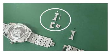
Onnect the remaining band links B and C.
