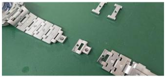
TRemove the pins from the link using tweezers or a pin puller, and separate the B link, C link, and pin.
