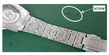
⑤While holding down the nearby links, remove the A link from the link you removed the screw from. If it is hard due to the adhesive, remove the A link by prying it up.
