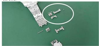
⑥Attach the Clasp link's C link with the B link on the bracelet side, and pass through the pin.
