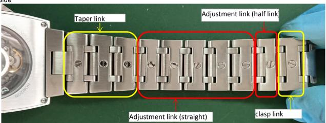
When adjusting the links, increase or decrease the links in the <u>red</u> frame area, and avoid removing the <u>yellow</u> frame area as much as possible. If you have to adjust it, put it back in place when you finish.
