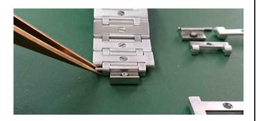
⑦Connect the clasp link's B link (with the clasp), to the clasp link's C link attached in step ⑥.
