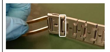
② After laying down the bracelet, confirm which part to be removed. To remove one link, remove two nearby screws.
