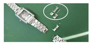
(9) Connect the remaining band links B and C.
