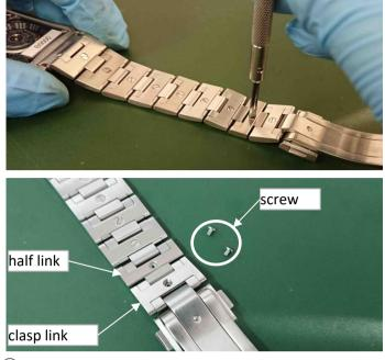
2Lift up the A link of the half link and clasp link to remove it.
