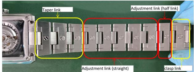
When adjusting the links, increase or decrease the links in the <u>red</u> frame area, and avoid removing the <u>vellow</u> frame area as much as possible. If you have to adjust it, put it back in place when you finish.
