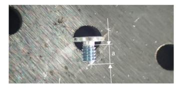
More than half of the entire thread should be coated. Threadlock adhesive amount  $\geqq a/2$
