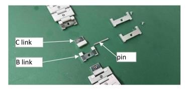
(8) Set aside the 5 parts (for one link): B link, C link, pin in (7), and A link screw removed in (4)(5).
