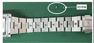
(5)While holding down the nearby links, remove the A link from the link you removed the screw from. If it is hard due to the adhesive, remove the A link by prying it up.
