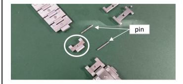
(4) Remove the connection (the half link's B link, C link) separated in (3), put aside the half link's A, B, and C links, pin and screws.
