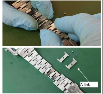
6 Separate the assembly of B link, C link, and pin.
