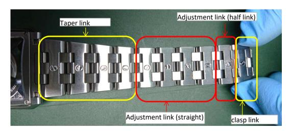
When adjusting the links, increase or decrease the links in the <u>red</u> frame area, and avoid removing the <u>vellow</u> frame area as much as possible. If you have to adjust it, put it back in place when you finish.
