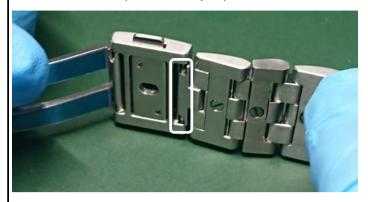
② After laying down the bracelet, confirm which part to be removed. To remove one link, remove two nearby screws.
