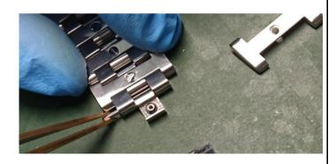
The clasp link's B link (with the clasp), to the clasp link's C link attached in step 6.
