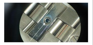
Apply it evenly inside the female thread. (In the photo A link was removed to make it easier to see)
