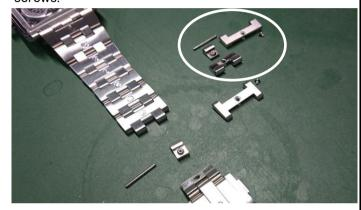
⑥Attach the Clasp link's C link with the B link on the bracelet side, and pass through the pin.
