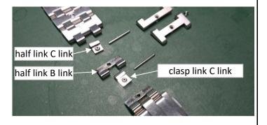
⑤Put aside the half link's A, B, and C links, pin and screws
