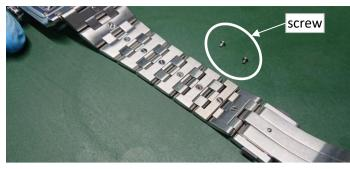
⑤While holding down the nearby links, remove the A link from the link you removed the screw from. If it is hard due to the adhesive, remove the A link by prying it up.
