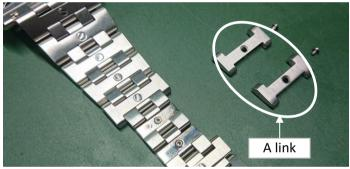
6 Separate the assembly of B link, C link, and pin.
