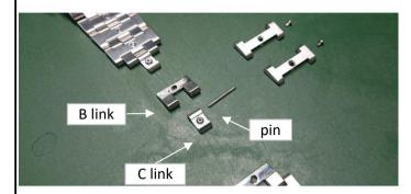
8 Set aside the 5 parts (for one link): B link, C link, pin in 7, and A link screw removed in 45.
