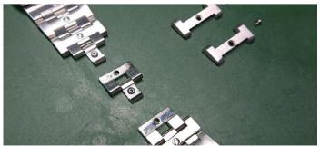
TRemove the pins from the link using tweezers or a pin puller, and separate the B link, C link, and pin.
